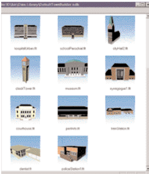
FIGURE 1 MultiGen-Paradigm's SiteBuilder 3D gives users a choice of object templates to assign to their existing point, line, or polygon features.
