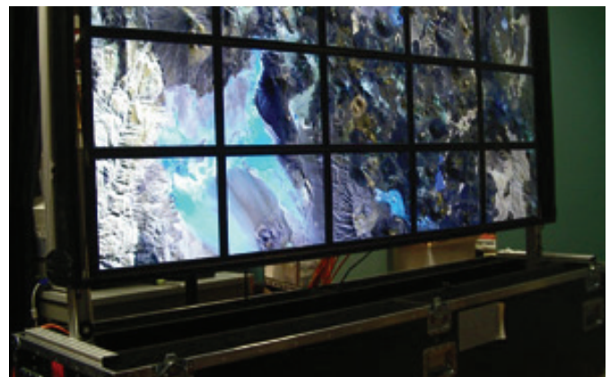
FIGURE 2 GeoWall II's 15-panel display contains 25 million pixels and, like the original GeoWall, supports stereoscopic visualization.
